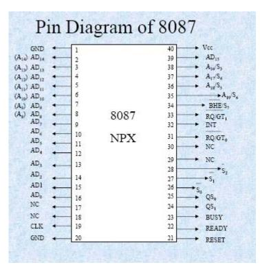
The 8088 and 8087 receive the same signals, CLK, READY, and RESET, from the 8284. This ensures that they are synchronized.
